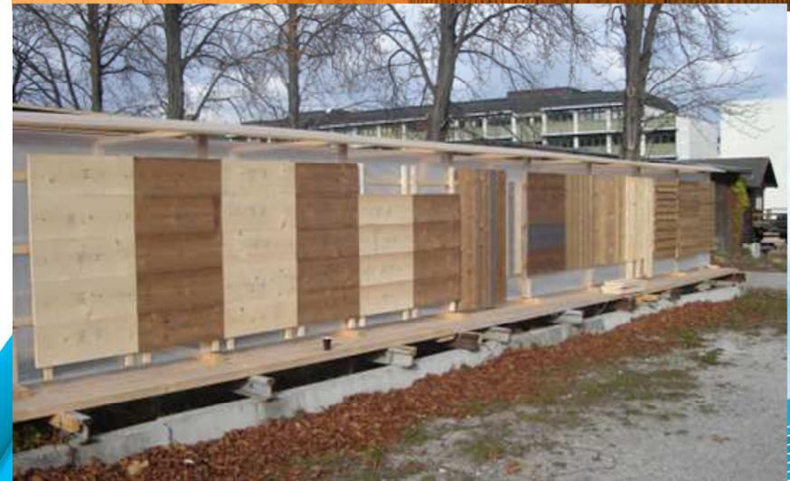
Facade elements differed in surface structure, sheathings, fixings and orientation
